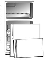
▲ WARNING — This appliance is designed to operate on a normal 115 volt, 15 amp, 60 cycle line. There should be a separate, grounded circuit serving this appliance only. Do not use an extension cord. Do not use any device that will alter the electrical performance of this appliance.
